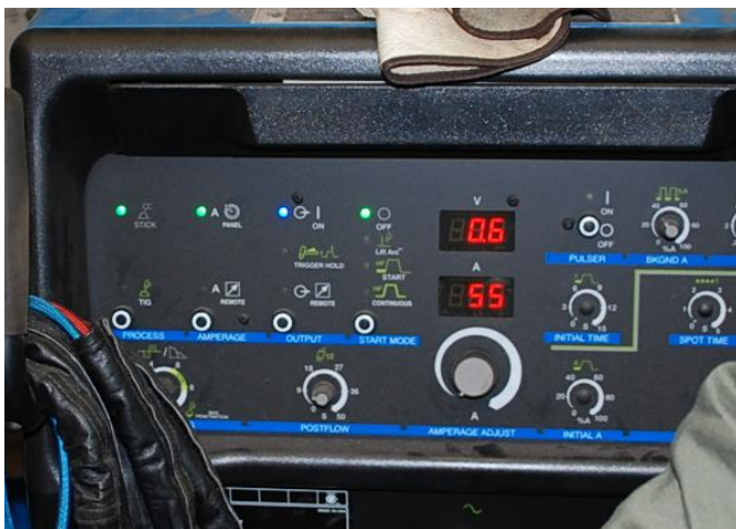
Figure 13 The voltage to current ratio confirms a resistance of 11 mOhm or less
