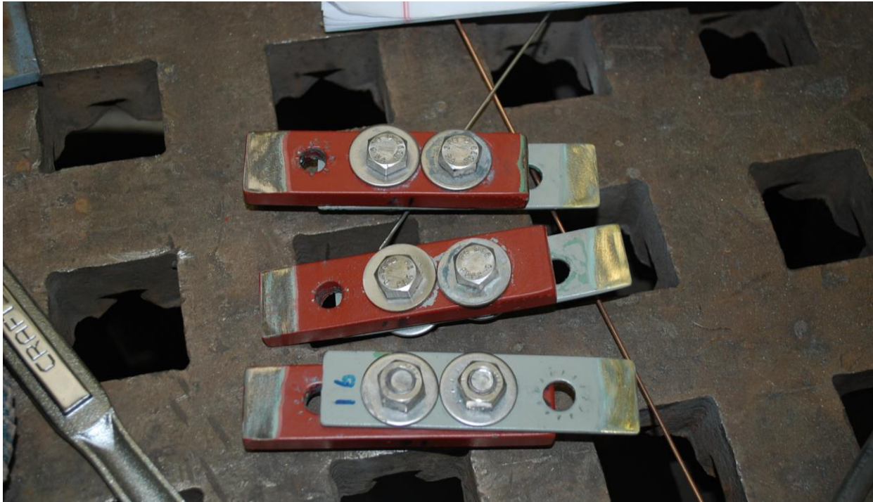
Figure 10 To prepare the samples, a small area on each end had the paint removed.
