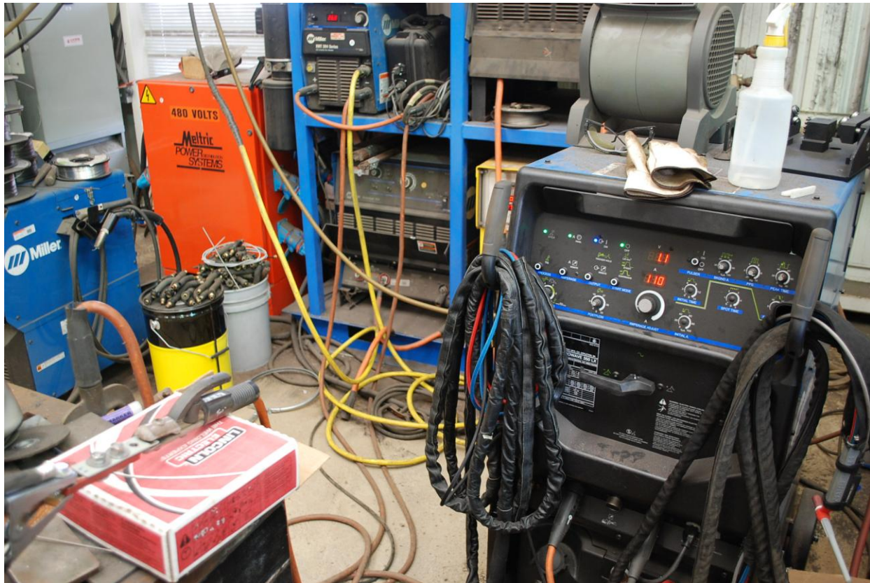
Figure 11 A Miller TIG Welding Machine, Syncrowave 350 LX was used to create the current.
