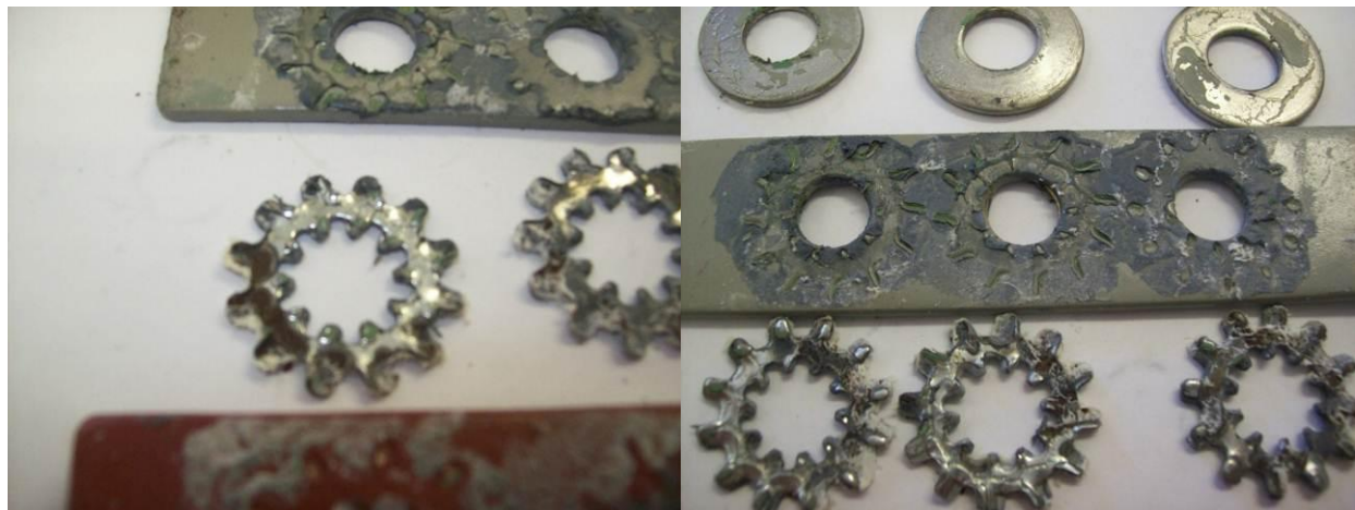
Figure 5 These non-stainless washers showed significant corrosion
