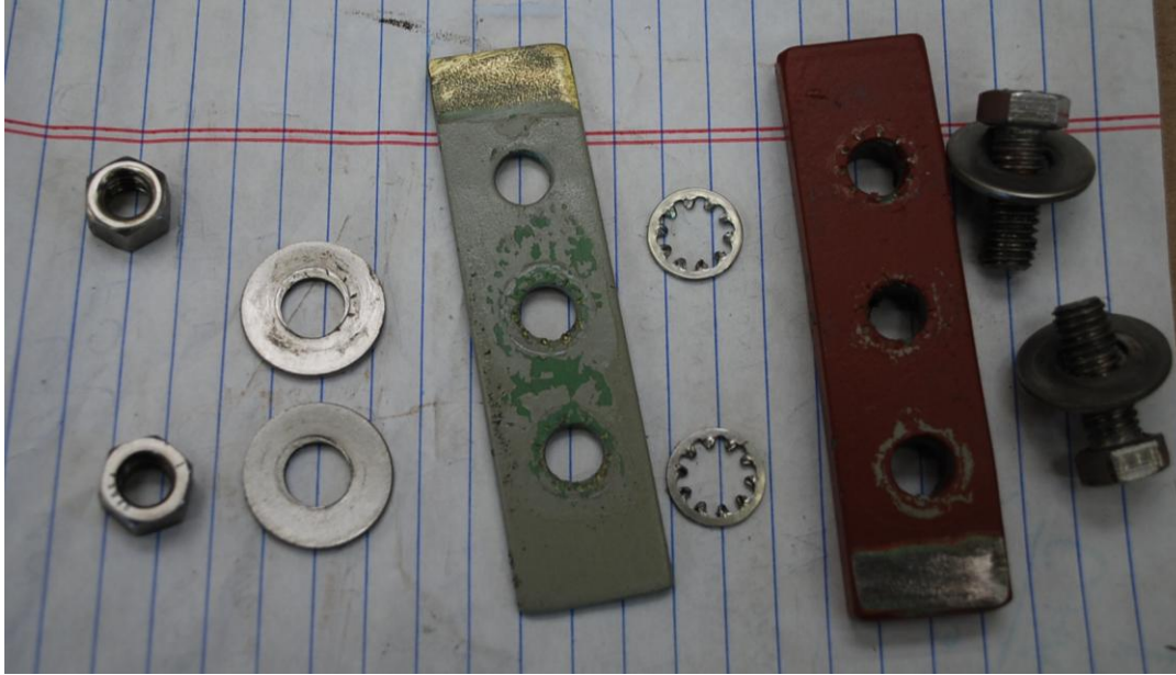
Figure 14 Sample 16 after testing. No damage at mating surfaces.
