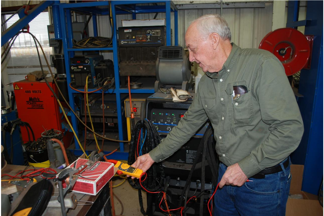
Figure 12 Ingalls Welding Engineer, Bennie Porter, verifies the current output with a Fluke 337 Clamp meter
