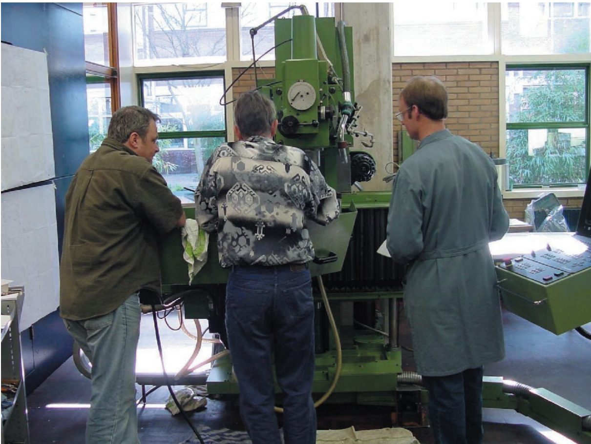
Milling of parts for the ATLAS Silicon Tracker.
