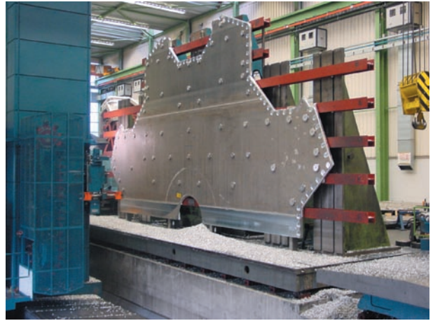
Figure 3.3: Final machining at Machinefabriek Amersfoort (IJsselstein) of a half Vacuum Vessel Endplate. Photo: courtesy Charles de Graaff, Schelde Exotech
