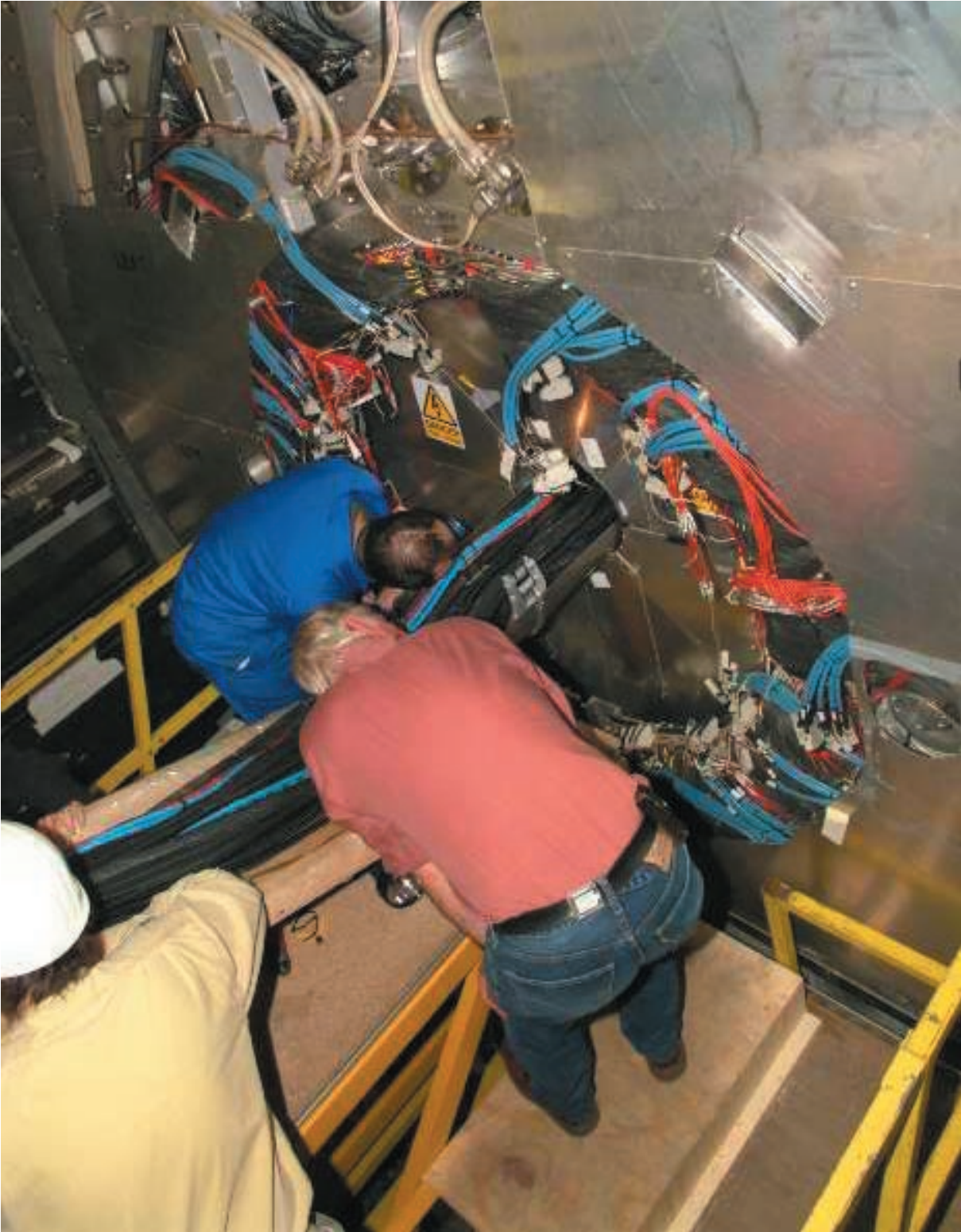
Installation of the Micro Vertex Detector (MVD) at ZEUS.
