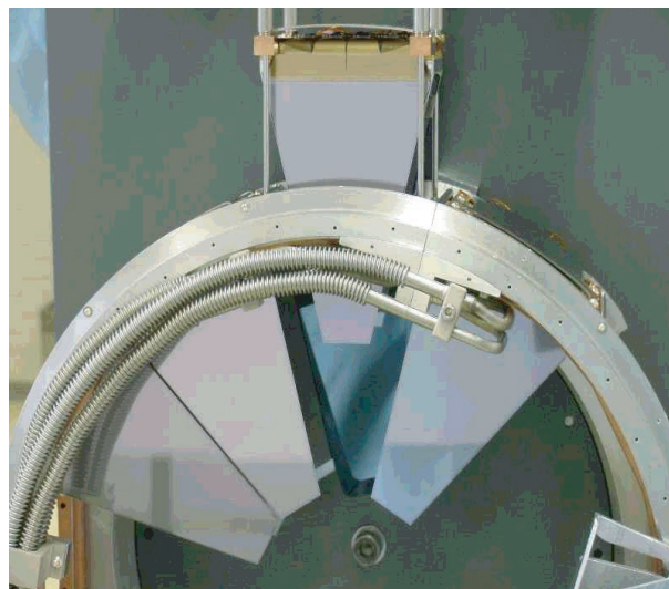
Figure 7.7: Installation of a detector module in the new wheel-shaped silicon detector ('Lambda Wheels'). The picture was taken during a test of the installation procedure in the NIKHEF workshop.
