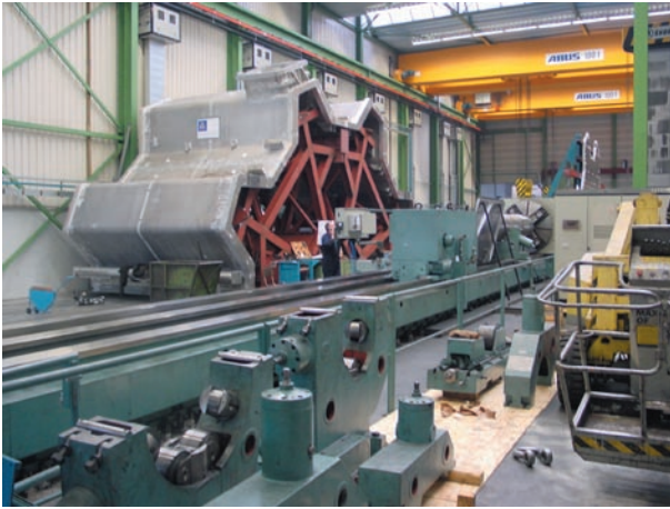
Figure 3.2: Half Vacuum Vessel Shell ready for final Machining at Machine Fabriek Amersfoort (IJsselstein). Photo: courtesy Charles de Graaff, Schelde Exotech
