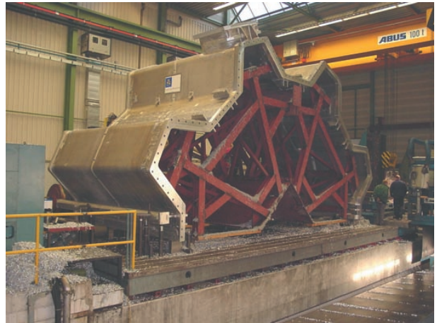
Figure 3.5: One of the ATLAS end cap toroids during the manufacturing stage. Photo: Courtesy Eddie Towndrow
