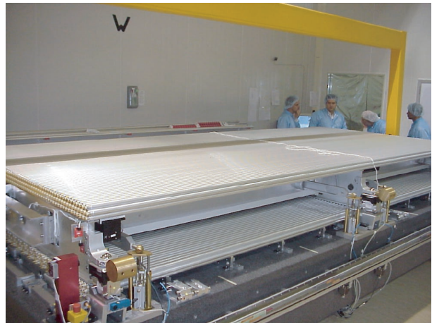
Figure 3.1: Photograph of the module-0 MDT chamber during the final assembly step.
