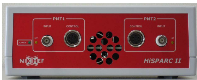
Figure A.1 – Front of the HiSPARC II electronics with connectors for the PMT control and signal cables for two channels.
