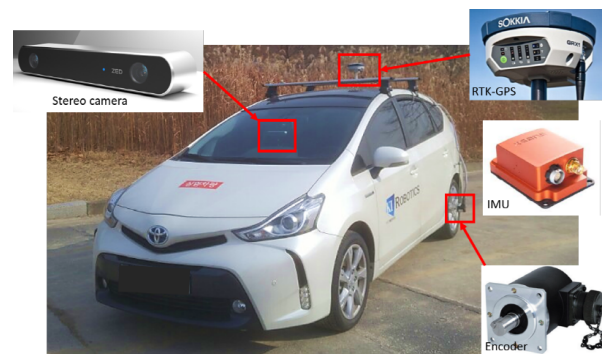
Fig. 3: The sensor system is equipped with a ZED camera, a MTi IMU, two wheel encoders and a RTK GPS. The RTK GPS is only used to initially set the direction and position of the vehicle at the start of the algorithm.
