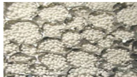
Amine based filter beads
