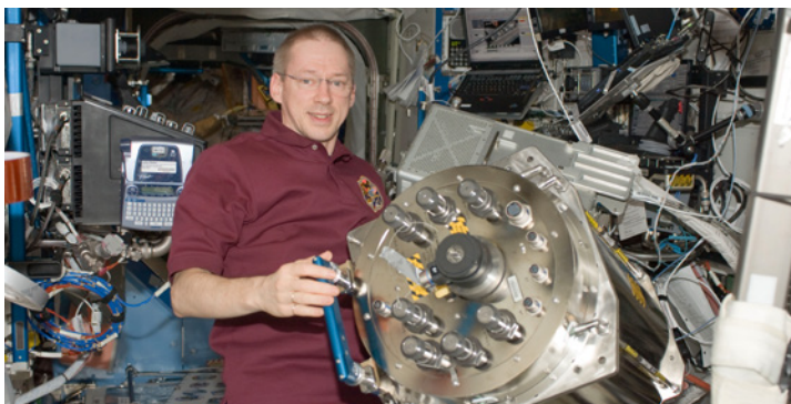
European Space Agency astronaut Frank De Winne exchanges the Distillation Assembly of the Urine Processor Assembly on the International Space Station which was designed and built at NASA's Marshall Space Flight Center. This device helps filter and purify crew waste in space, conserving more water and reducing the amount of resupply the astronauts require from Earth. (NASA)
