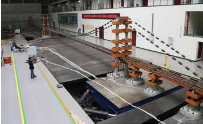
The scale model of the Taizhou Bridge in the Tongji MFST lab.
