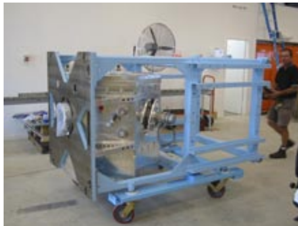
GSAOI cryostat being transported in its partially filled integration frame after fit check
