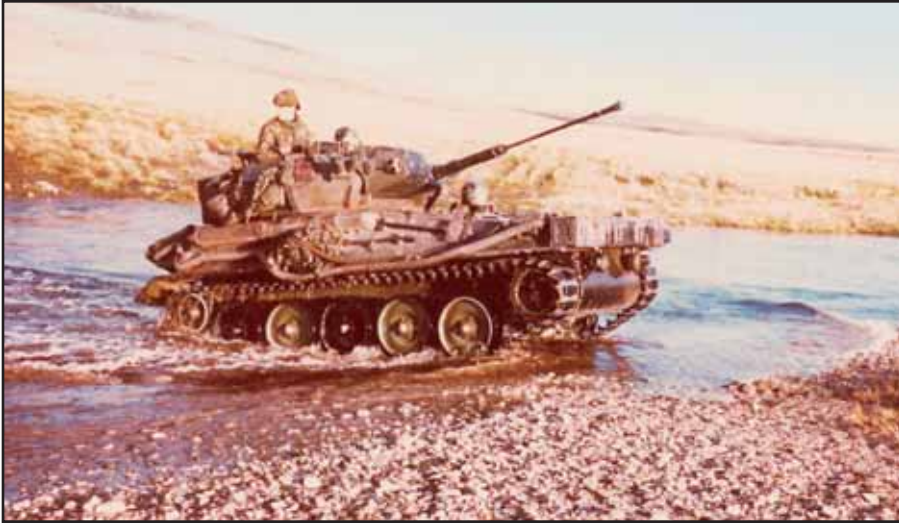
"...the 'Scimitar,' which was built on the same chassis as the Scorpion, weighed about the same, and mounted a high-velocity 30mm Rarden cannon. The 30mm fired armor-piercing, discarding sabot (APDS), high-explosive, and an armor-piercing special-effect (APSE) round, which could easily penetrate an infantry fighting vehicle or armored carrier."
