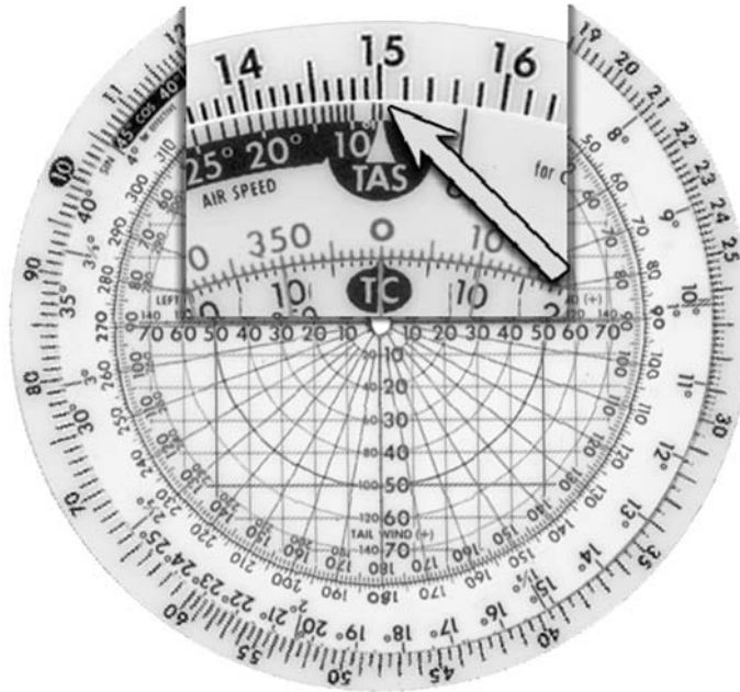
Figure 4.6-5 In-Flight Wind Calculation 1
