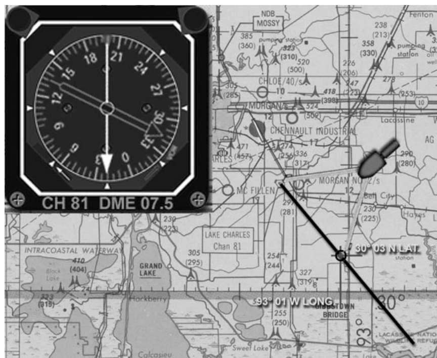
Figure 4.2-24 TACAN Position Fixing
