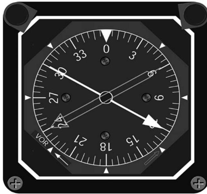
Figure 4.1-3 Remote Gyro Vertical Compass Card
