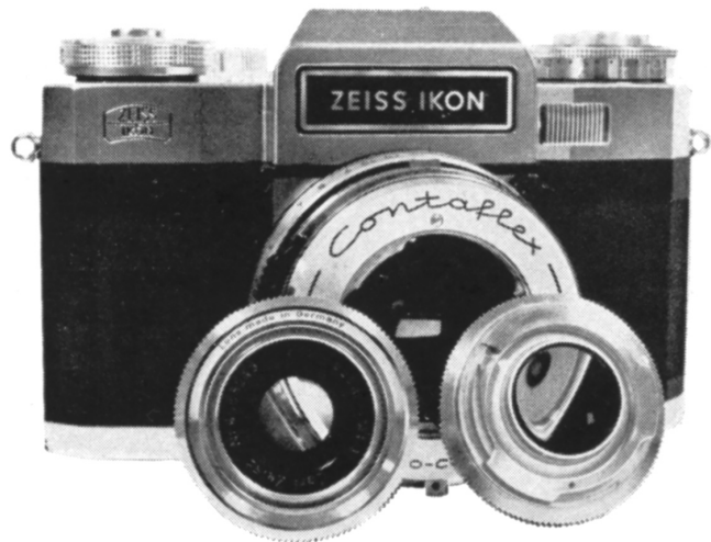
Life-size images may be made with Contaflex camera by switching front component of normal lens with Pro-Tessar M 1:1 Accessory. Metering is unaffected.
