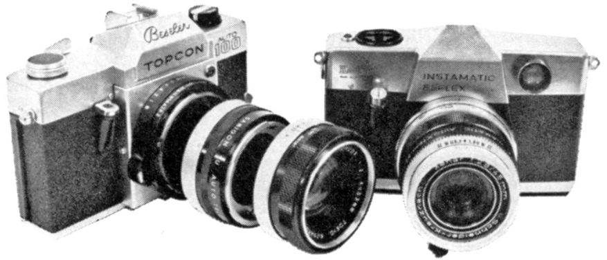
Telephoto extenders, available for some LSR's, fit between lens and its shutter housing. It doubles the lens's focal length, without altering its minimum focusing distance, thus permitting tighter framing. Model shown on left is the Samigon, the one on right, Accura. Similar units are also available from other suppliers.
