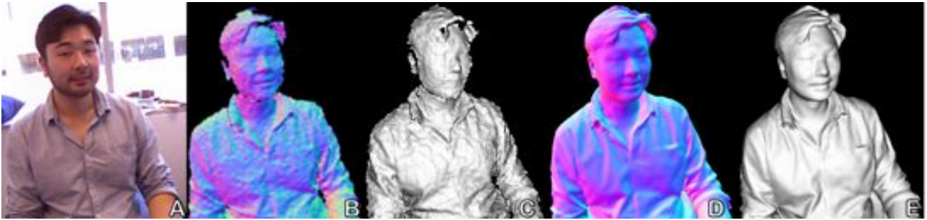
Figure 2: RGB image of scene (A). Extracted normals (B) and surface reconstruction (C) from a single bilateral filtered Kinect depth map. 3D model generated from KinectFusion showing surface normals (D) and rendered with Phong shading (E).
