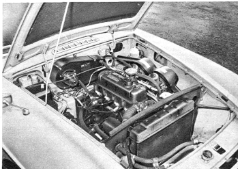
The engine compartment is tidily arranged, and the bonnet lined with sound-deadening material. Flexible pipes passing around the radiator are to and from the engine oil cooler, out of view here
