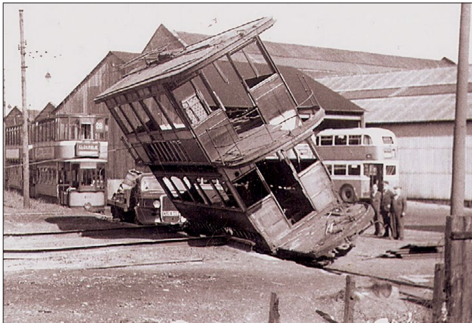
Now devoid of all reusable parts, the shell of a Standard tram is pulled over at Elderslie Depot prior to burning.
