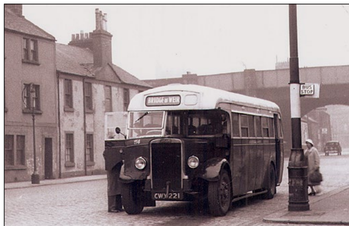
Garner's 51 (CWY 221), a Leyland Tiger TS8 with Leyland 35 seat rear entrance body, was originally in the Todmorden Corporation fleet and came to Garner from Baxter of Airdrie. Here it lies over in Abercorn Street, Paisley, before returning to Bridge of Weir.
