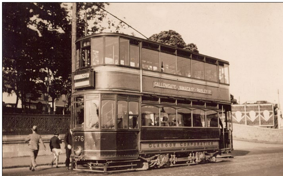
Modernised Standard tram 276 still operates with a trolley pole in 1929 and displays an unusual lapse in having a blank "via" screen. The new 8'-0" wheelbase truck retains a tie-bar below the main side truck frame – a very short-lived feature. Had this view come to light in time, it would have been included in the book. (STTS Collection)
