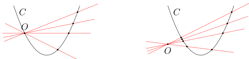
Figure 14.5: Projection from a point on the conic and from a point not on the conic respectively.
