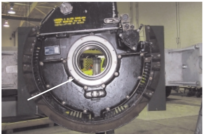
Pump housing rear lip seal.
