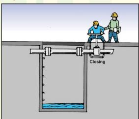
**Example 2:** Removing any generator that may produce toxic gases
