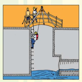
The responsible person shall provide and inspect all equipment (like resuscitators) and personal protective equipment (like approved breathing apparatus, safety helmets, protective clothing, safety harnesses and rescue ropes). An employer shall also be responsible for providing training to ensure that the workers understand clearly how such equipment and tools are to be used.
