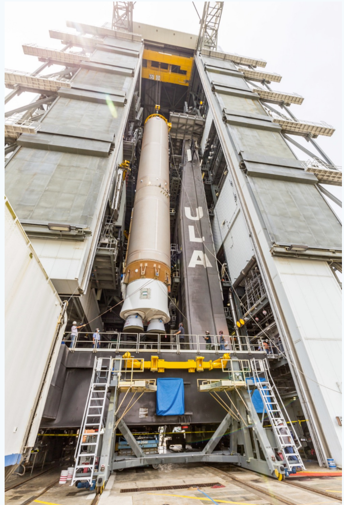
United Launch Alliance hoists its Atlas V first stage onto the mobile launch platform at Launch Complex 41, Cape Canaveral Air Force Station, about a month and a half before Perseverance is set to launch. Image Credit: ULA
