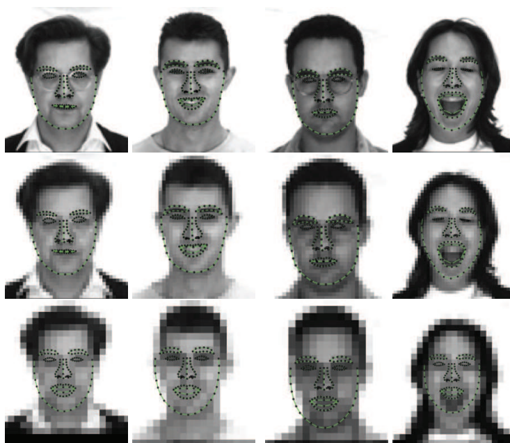
Figure 11: Shape detection examples at different resolutions. Note how the shape estimation is almost as good regardless of the resolution of the image.
