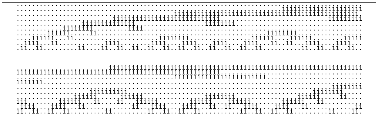
Figure 14.10-B: The length-10 binary strings with no substring 1xy1 (where x and y are either 0 or 1) in minimal-change order. Dots denote zeros.
