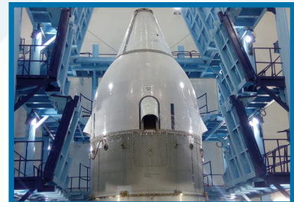
CES Ground Resonance Test
