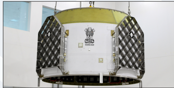
Crew Module Fairing with Grid Fins
