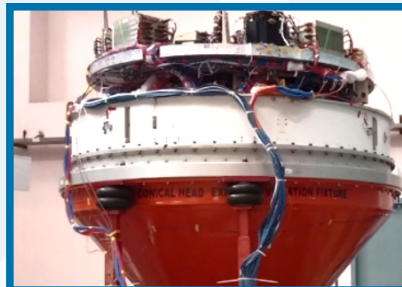
Equipment Bay vibration test
