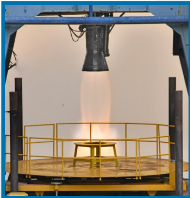
AR 6 VIKAS Engine hot tests
