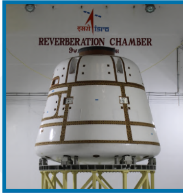
Crew Module Acoustic Test at ISITE, URSC
