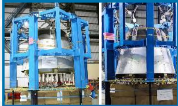
Crew Escape System separation test
