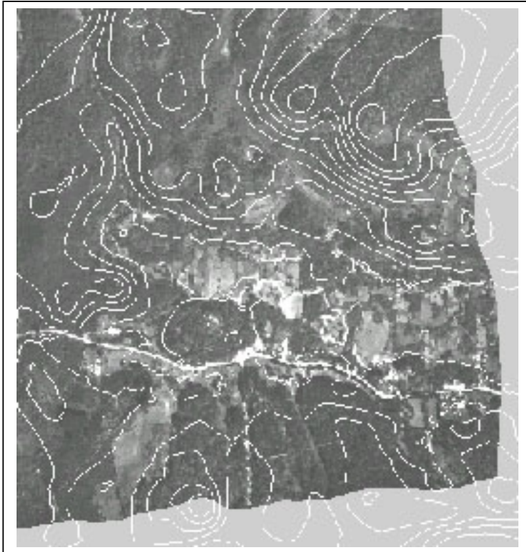
Figure 8: orthophoto with overlay of automatic generated contour lines
