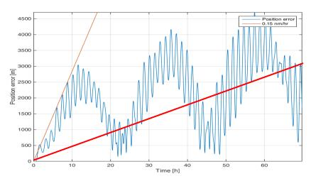
The figure shows such long time behavior of a free inertial navigation (example: data obtained from iNAT-RQT over more than 3 days): Link
