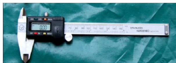
Fig 2: Electronic Digital Calliper used for the study.
