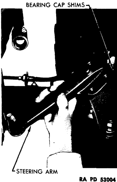
Figure 161—Removing Steering Arm
