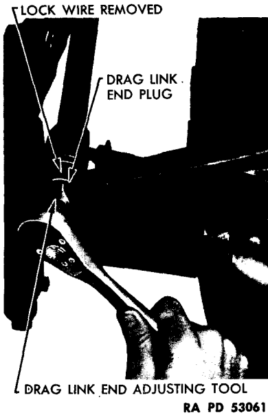
Figure 190—Adjusting Drag Link End
