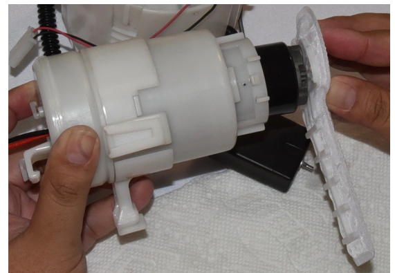
Install the Hondata low pressure fuel pump and fuel filter sock
