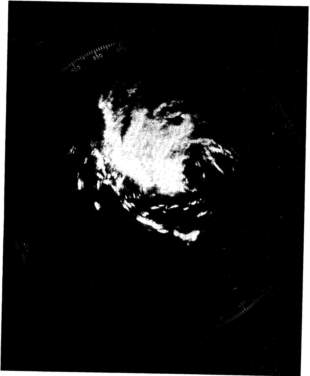
Figure 11. Radar picture of Severe Tropical Storm Agnes taken at 5.00 a.m. on 30 July 1978. (Range markers at 40-mile intervals)
