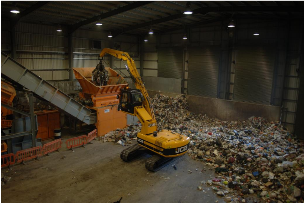
Fig 25 shows an internal view of the New Earth Solutions MBT facility at Cotesbach, Leicestershire. This facility has a throughput of 50ktpa 67 .
