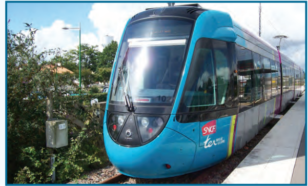
Tram-train : A hybrid train used in parts of Europe, able to run on normal electrified rail lines and also in ‘tram’ mode on street enabling lower cost extension of rail services. Could work well in Cardiff to link City and Coryton lines to Cardiff Bay and beyond, as well as potential extension to the North West of Cardiff and RCT. The best known example is Karlsruhe in Germany. Currently being trialled in Sheffield.
