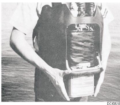
**Figure 5-18. Inserting the canister.**
