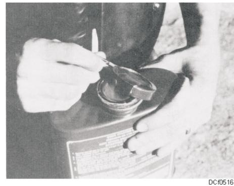
Figure 5-16. Step 5, removing the tear-off cap.
