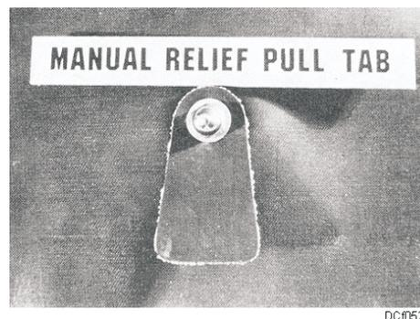
Figure 5-23. Manual relief valve tab.
