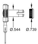
TUNING MACHINE THRU-HOLE INNER DIAMETER .734"
