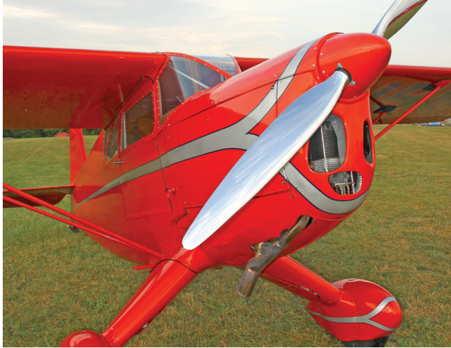
The 95-hp, four-cylinder, inverted, air-cooled Cirrus engine gave the airplane a distinctive look.
