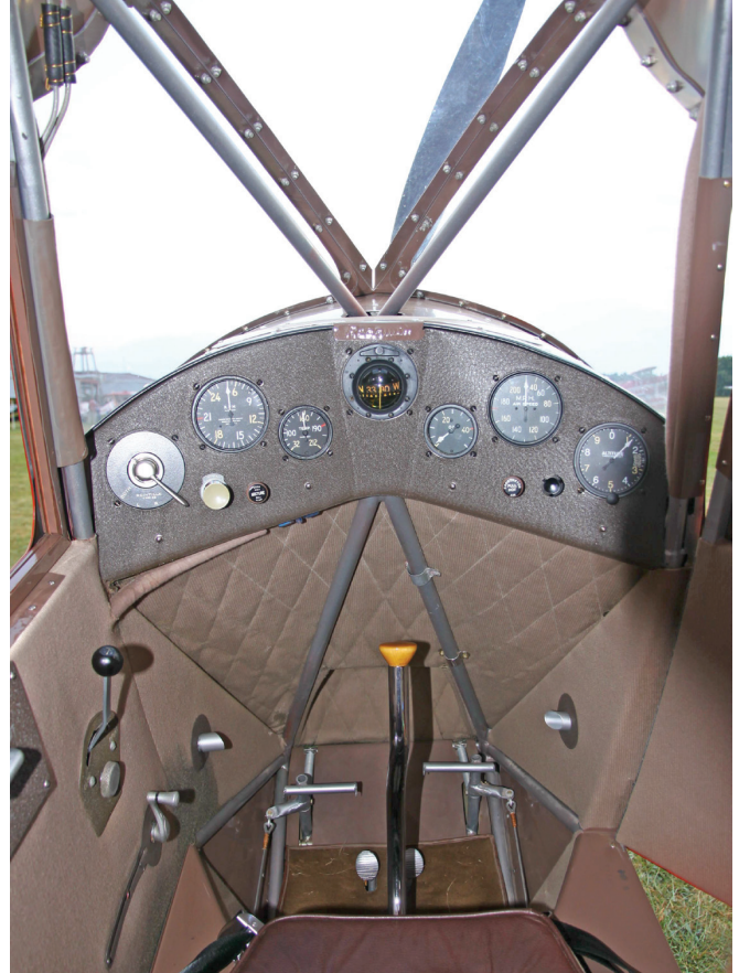
The pilot's view to either side of the nose was excellent and the instrumentation minimal.
