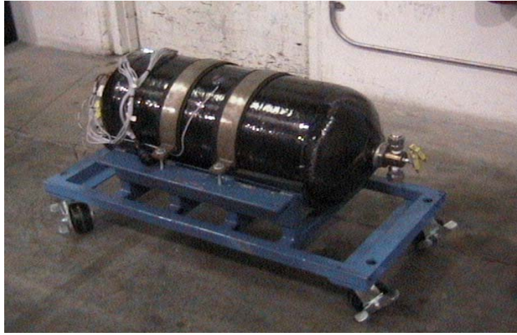
Figure 15. Prototype Ovonics solid state hydrogen storage system
