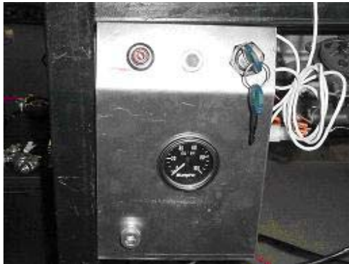
Figure 3. Engine dashboard which houses ignition switch, starter button And oil pressure gauge
