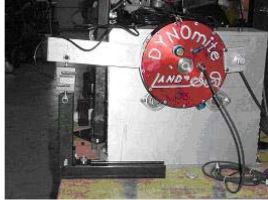
Figure 5. Timing window placed on flywheel cover
