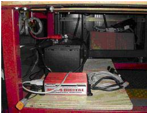
Figure 7. Battery and ignition relocated underneath the cart
