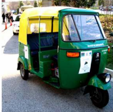
The Indian Bajaj three-wheeler single-cylinder i.c. engine taxi converted by Energy Conversion Devices from compressed natural gas fuel to hydrogen
