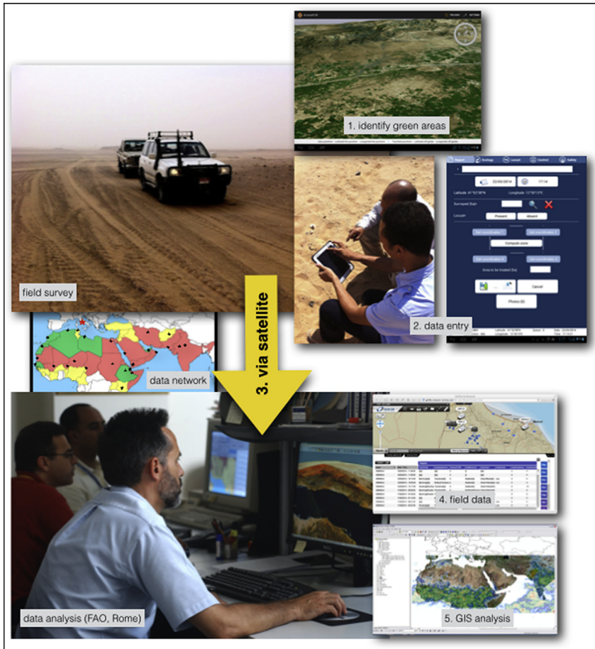
FIGURE 4.2.11 The flow of data used for desert locust early warning in which data are collected during field surveys, immediately entered into eLocust3 and transmitted by satellite in real time to national locust centers and the FAO Desert Locust Information Service in Rome where analyses are undertaken using a custom geographic information system (GIS) in order to provide assessments, forecasts, and early warning.
