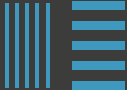
MASK (4X8) VERTICAL: PITCH 200 CD 74 HORIZONTAL: PITCH 400 CD 164
