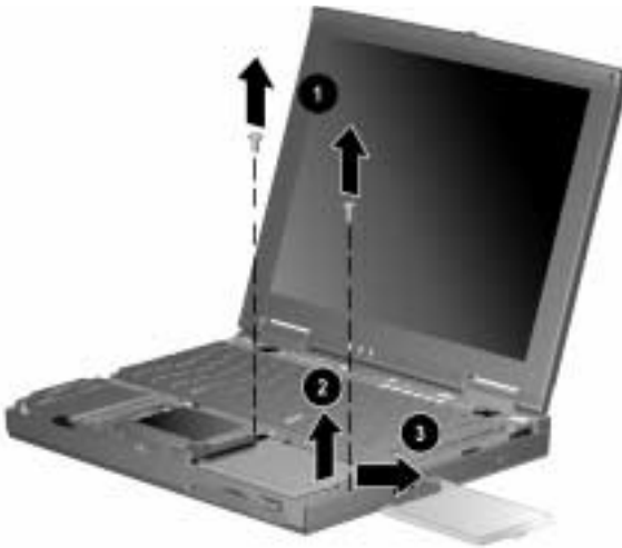
Figure 5-17. Removing the Hard Drive
