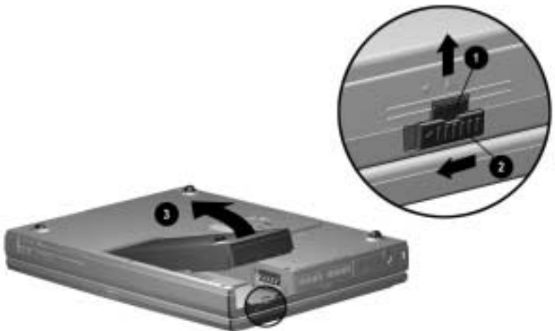
Figure 5-2. Removing the Battery Pack
