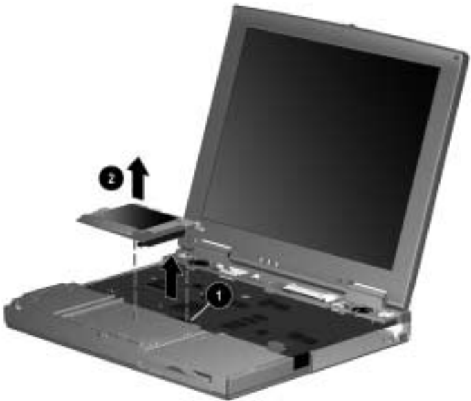
Figure 5-22. Removing the TouchPad
