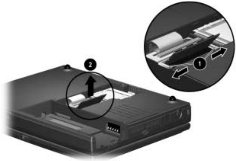
Figure 5-13. Removing a Memory Expansion Board
