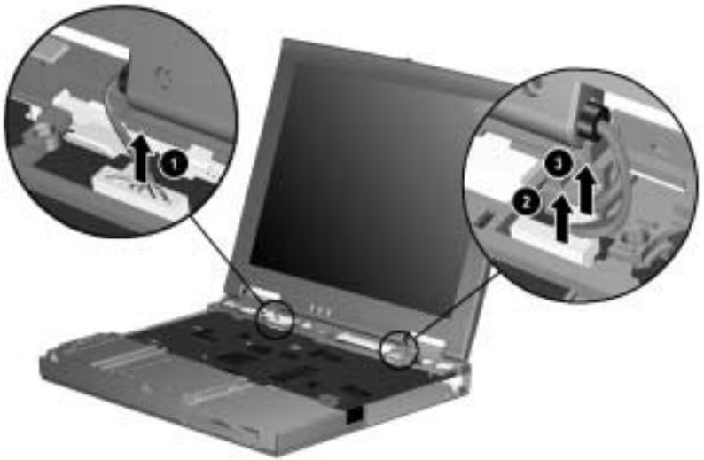
Figure 5-25. Disconnecting the Display Cables
