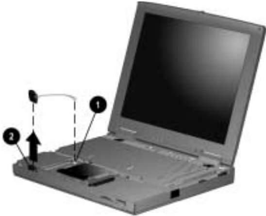
Figure 5-18. Removing the RTC Battery
