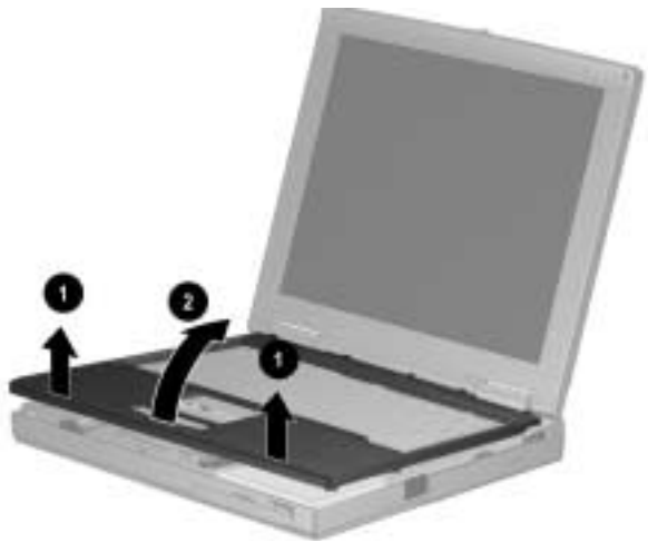
Figure 5-16. Removing the Top Cover
