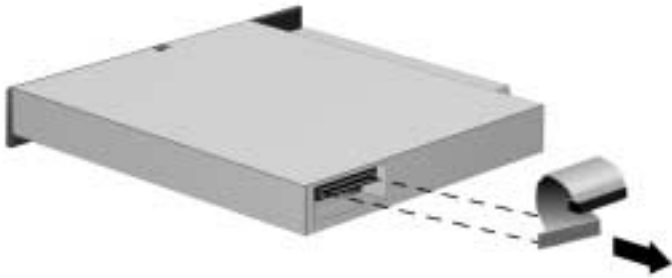
Figure 5-9. Removing the CD-ROM Drive Cable
