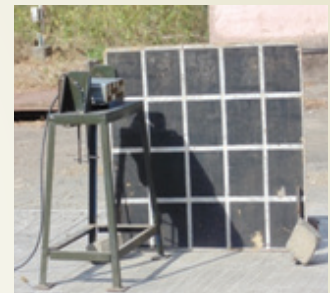
Figure 24. Test Set-up for Ejection Velocity
