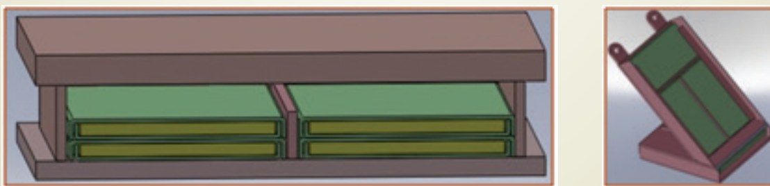
Figure 6. Internal Configuration of Reactive Elements of ERA Mk-II
