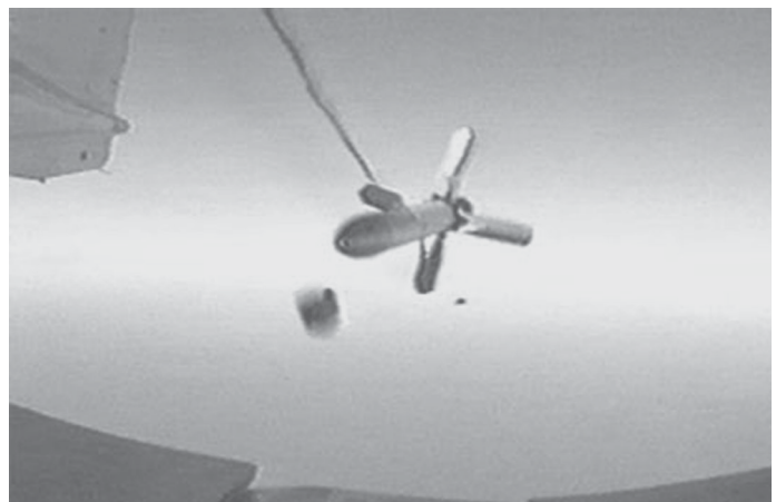
The Integrated Defensive Electronic Countermeasures Block II, consisting of both an onboard jammer and a towed decoy, enhances aircraft survivability against radio frequency-guided missiles.
