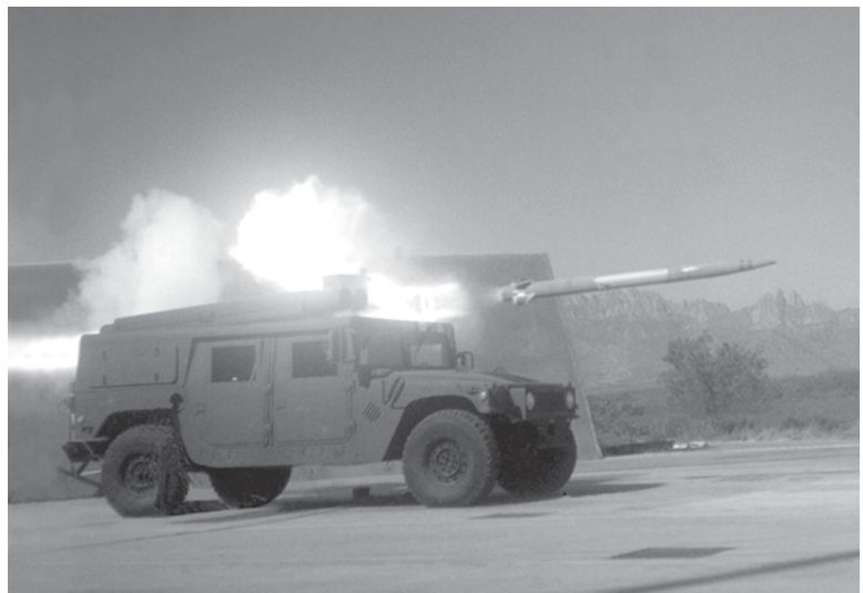
The Line-of-Sight Anti-Tank Missile uses kinetic energy as its kill mechanism and is the first of the Army's Kinetic Energy Missile programs.
