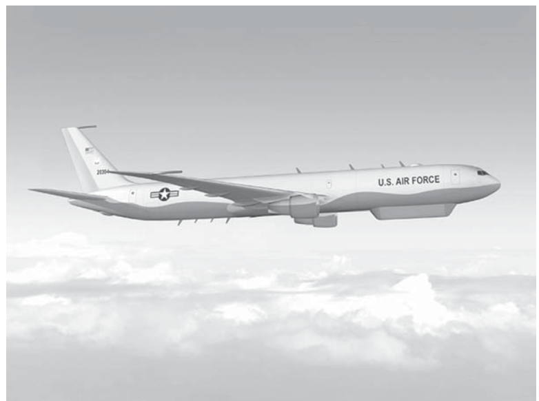
The Multi-sensor Command and Control Aircraft, recently designated the E-10A, is intended to meet the Air Force's need to integrate Command and Control Intelligence, Surveillance, and Reconnaissance, and Information Warfare functions on a single platform.
