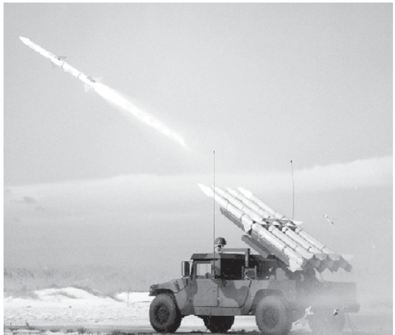
The Surface-Launched Advanced Medium Range Air-to-Air Missile system intends to give the Army the capability to engage targets beyond line-of-sight and at greater ranges than the Stinger-based systems.
