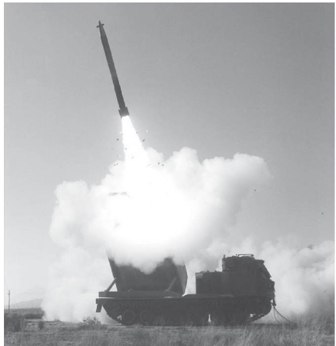
The Guided Multiple Launch Rocket System consists of two variants of rockets fired from the M270A1 or High Mobility Artillery Rocket System launchers.
