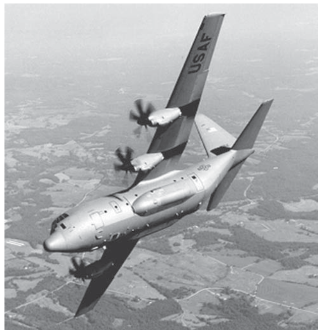
The C-130J is a medium-range, tactical airlift aircraft designed primarily for the transport of cargo and personnel within a theater of operations.
