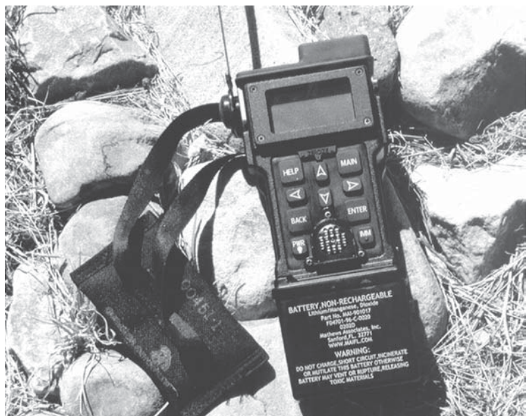
The Combat Survivor Evader Locator includes hand-held radios, unmanned base stations, and rescue center workstations.
