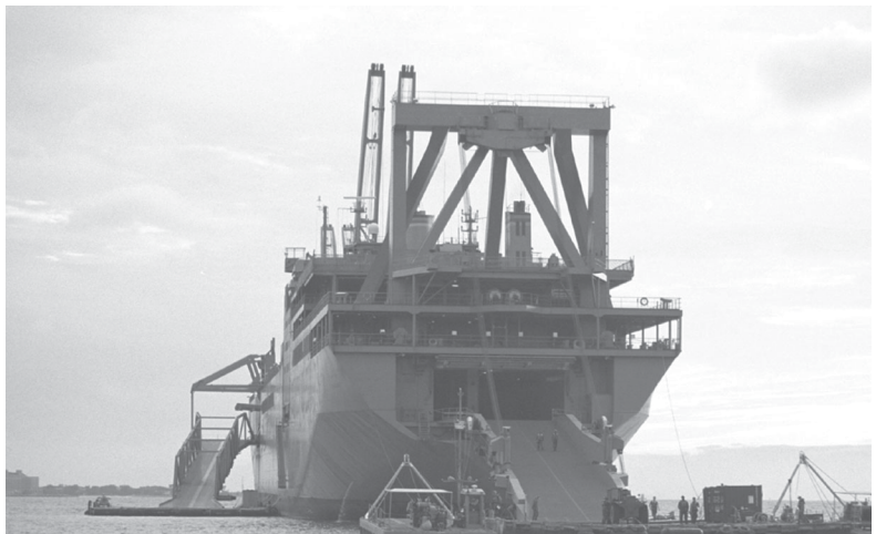
The sealift ships are capable of self-sustained roll-on/roll-off and lift-on/lift-off operations at a pier and at anchorage.
