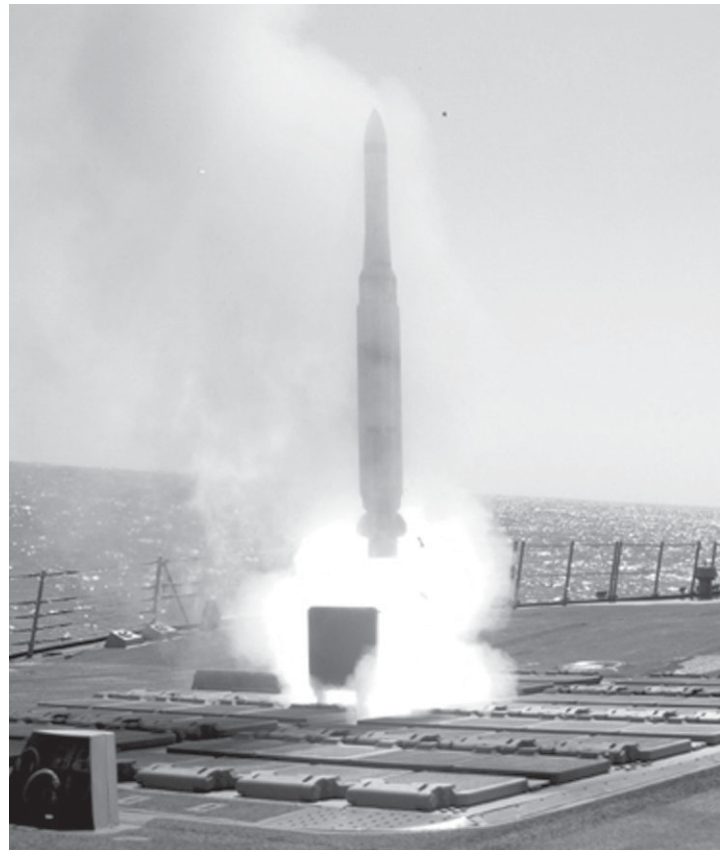
On Aegis ships, the Evolved Seasparrow Missile will be launched from the Mark 41 Vertical Launch System.
