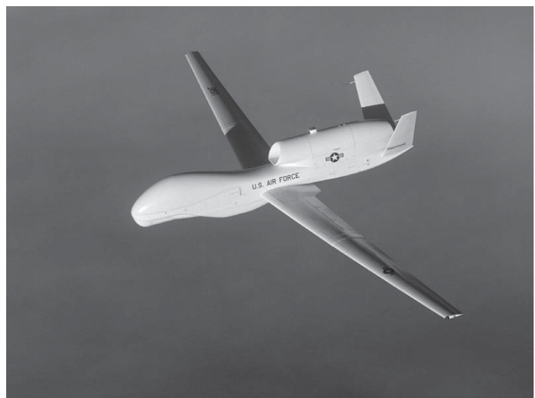
The Global Hawk UAV system comprises an air vehicle component with air vehicles, sensor payloads, avionics, and data links.
