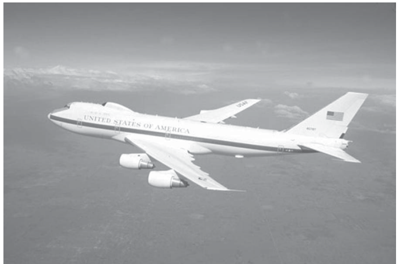
The E-4B is a militarized Boeing 747-200 aircraft that provides a survivable national airborne operations center for senior leadership.
