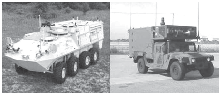
Both versions of the Joint Services Light Nuclear, Biological, and Chemical Reconnaissance System will be employed in forward combat areas and integrated into NBC reconnaissance, surveillance, monitoring, and survey plans to detect chemical or biological attack.
