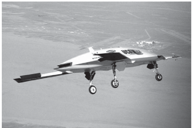
The maximum altitude demonstrated was 35,000 feet and a top speed of 250 knots.
