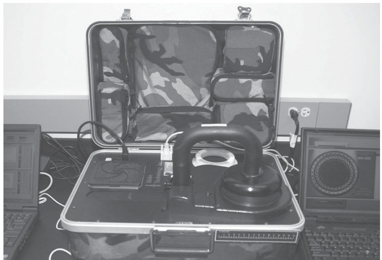
The Joint Biological Agent Identification and Diagnostic System is intended for use by military clinicians and other trained personnel to screen for biological agents given such factors as known or suspected threat agents and geographical endemic diseases.
