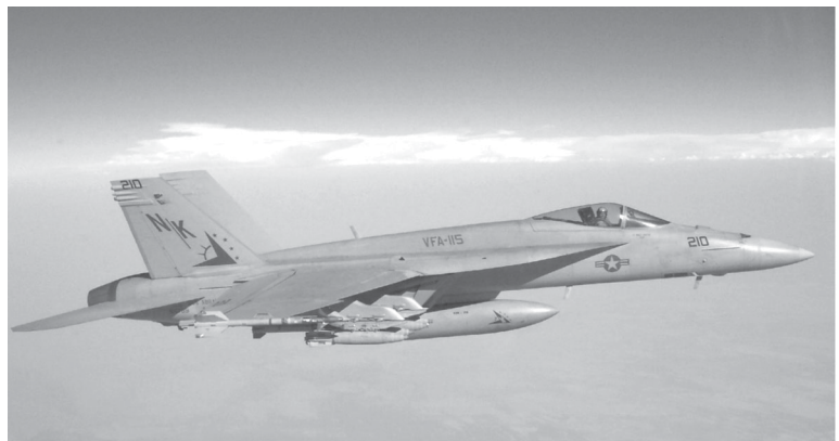
The FA-18E/F Super Hornet is a multi-mission, day/night strike fighter aircraft that provides precision strike capabilities to Joint Task Force and Carrier Strike Group Commanders. The F/A-18E is a single-seat aircraft while the F/A-18F is a two-seater. The EA-18G is the planned electronic attack variant and will closely resemble the two-seat F/A-18F model.
