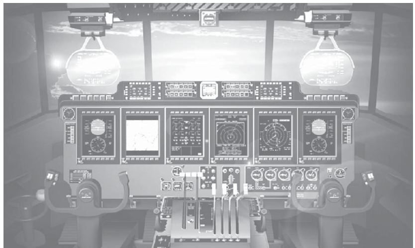
The C-130 Avionics Modernization Program upgrades the cockpit by replacing aging, unreliable subsystems, and adds equipment necessary to meet navigation and safety and Global Air Traffic Management requirements.
