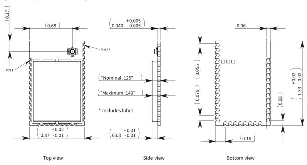
The drawings below show the XBee through-hole model
