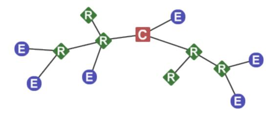
Note Each Zigbee network must be formed by one, and only one, coordinator and at least one other device (router or end device).
