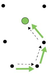
After obtaining a source route, the data collector sends a source routed transmission to the remote device.
