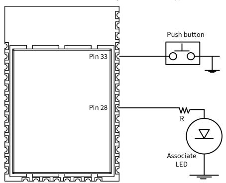
A pushbutton and an LED can be connected to the XBee/XBee-PRO Zigbee RF Module pins 33 and 28 (SMT), or pins 20 and 15 (TH) respectively to support the commissioning pushbutton and associate LED functionalities.
