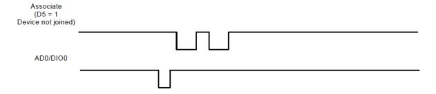
The following image illustrates the behavior pressing the button once on a remote device, causing a broadcast node identification transmission to be sent. All devices that receive this transmission blink their associate pin rapidly for one second if the associate LED functionality is enabled (**D5** = 1).
