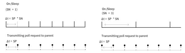
Setting SN > 1 allows the device to silently poll for data without asserting On/Sleep. If RF data is received when polling, On/Sleep will immediately assert.
