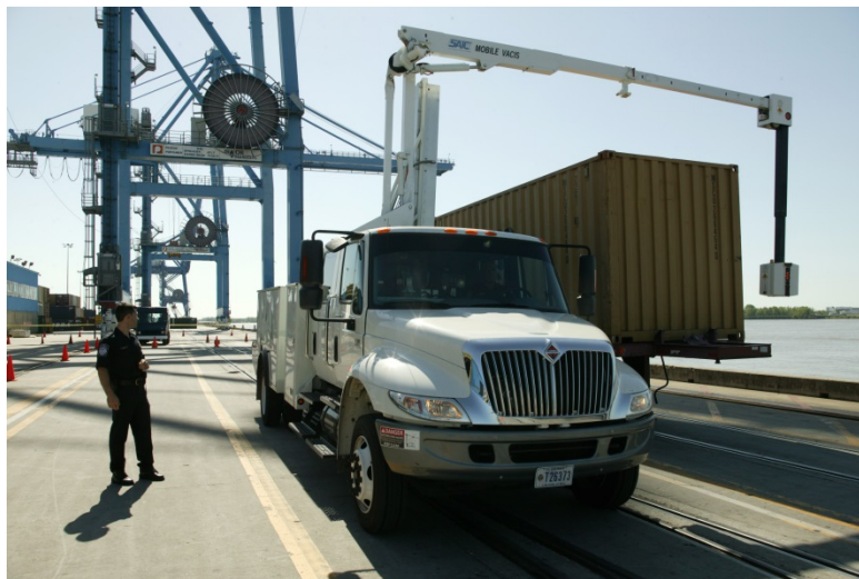
A Radiation Portal Monitor is used to inspect a shipping container for contraband.
