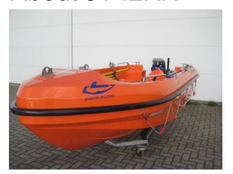
The JY42KR rescue boat is design and built according to the IMO "International Convention on Safety of sea 1974" and all its update amendments including the 1996 revision of Chapter III and the inception of the associated International Life-saving Appliance Code (LSA CODE). Every test meets the requirements about rigid rescue boat of IMO "Life-saving Appliances Test" and IMO Resolution MSC.81 (70).
