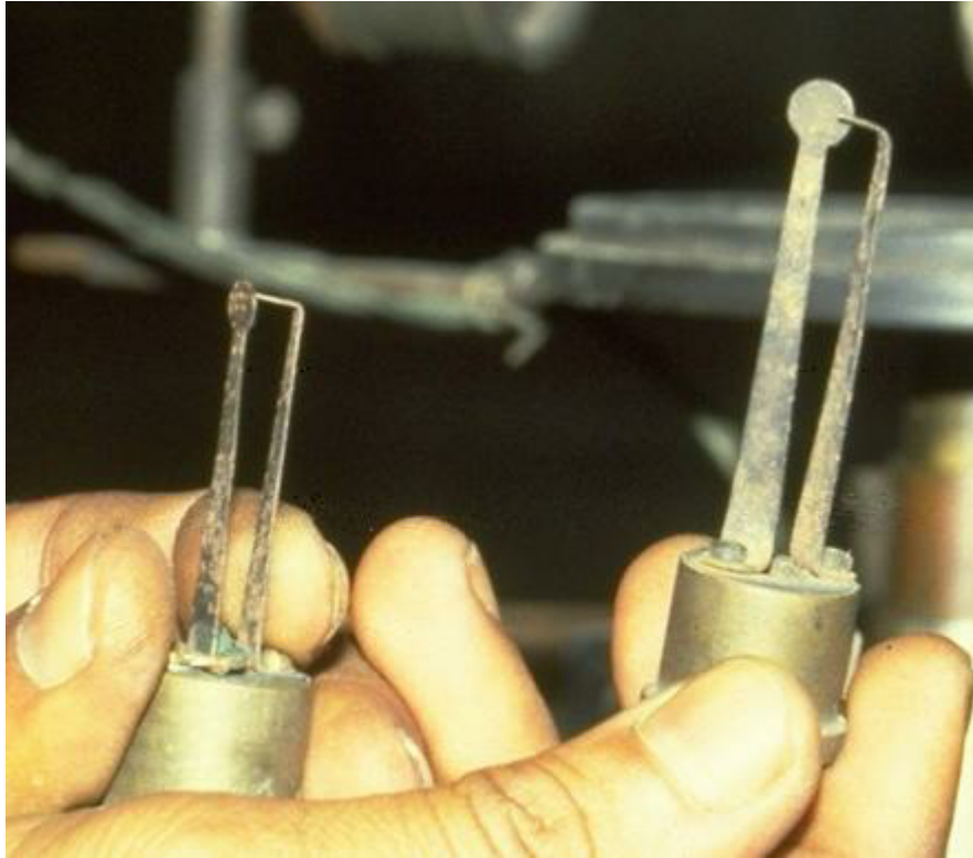
Figure 5. Two of Bose's point contact detectors, removed from the receiving antennas.
