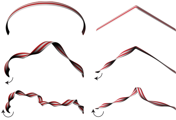
Figure 5: Asymmetry of twist: anisotropy of the cross-sections and natural curvature of the centerline “conspire” to produce non-uniform twist distribution. From top to bottom: reference configuration, moderate twist, large twist.
