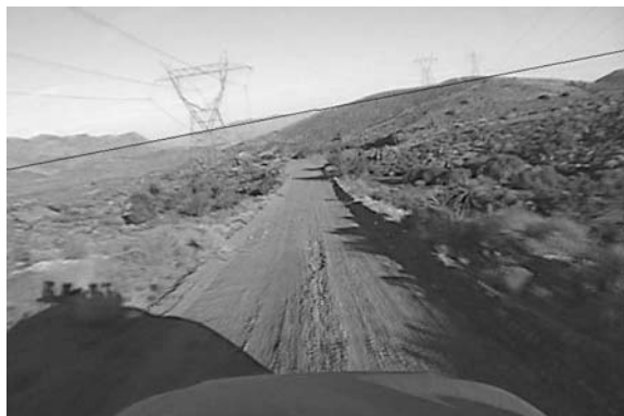
Figure 7. Output of horizon detector is the dark line.
