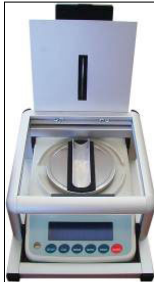
Figure 2. The custom 0.7 mm guillotine mounted above the snippet weighing balance. The image shows the underside of guillotine slot and collection trough on the balance.
