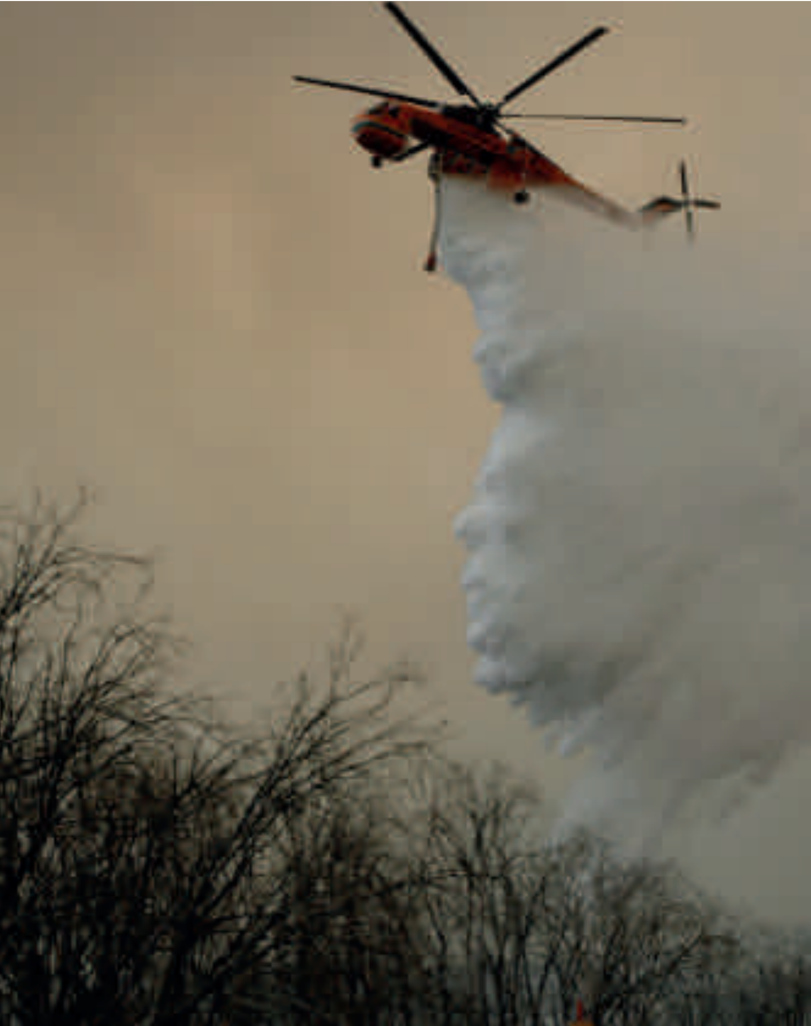
Figure 17: Elvis – the Erickson Air-Crane fire bomber – dumping about 9,000 litres of water to assist firefighters at Falls Creek, Victoria. Specialised firefighting aircraft like this are loaned for the bushfire seasons in both the Northern and Southern Hemispheres each year. Such aircraft are expensive to operate.
