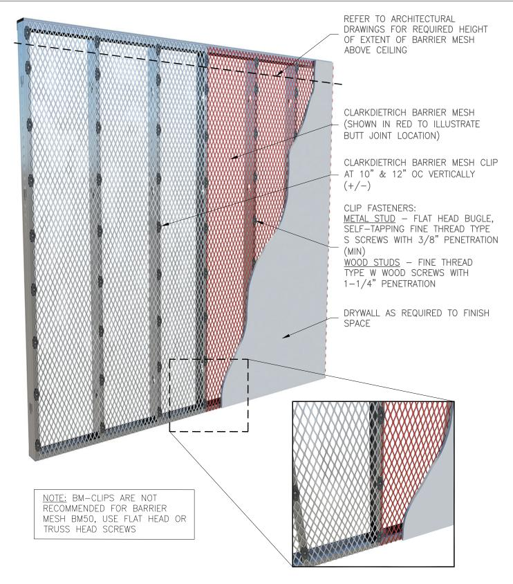
BARRIER MESH & BARRIER MESH CLIP LAYOUT
