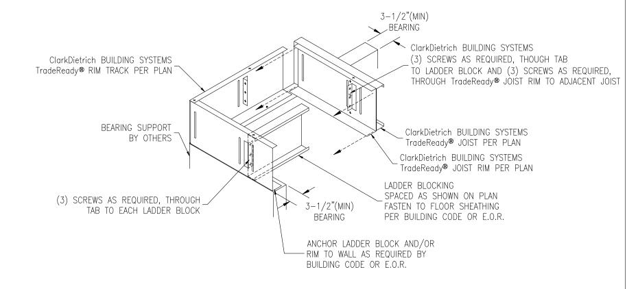
F2205 LADDER BLOCKING — RIM—BACKED JOIST ClarkDietrich TradeReady Floor Joist System
