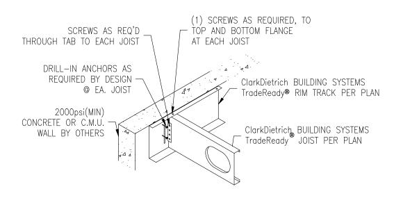
F1113 JOIST RIM — CMU WALL — BALLOON ClarkDietrich TradeReady Floor Joist System
