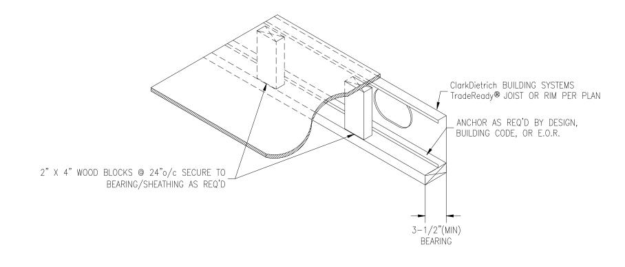
JOIST - RIM - FRAMING PARALLEL TO WALL
